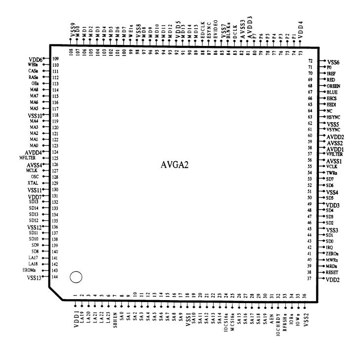
144 PIN PQFP pinout
